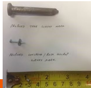
Left: subsidence monitoring markers for foreshore tree's (top) or rock/concrete (bottom)
